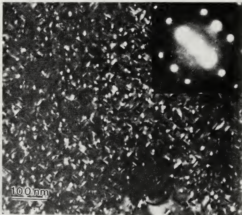
Figure 11B Dark-field TEM Micrograph of 6061 Aluminum Aged for 3000 Seconds at 473K.
